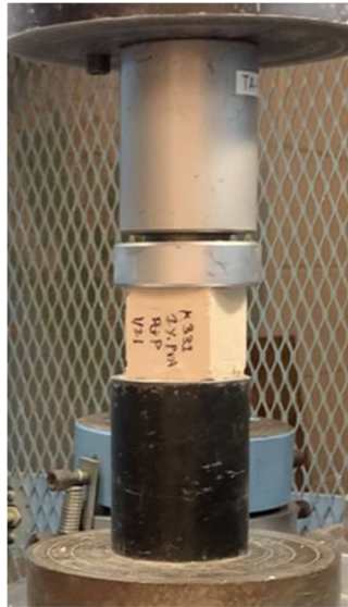
Figure 8. Compressive strength test experimental setup.
